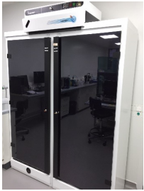
Chemical storage cabinets
